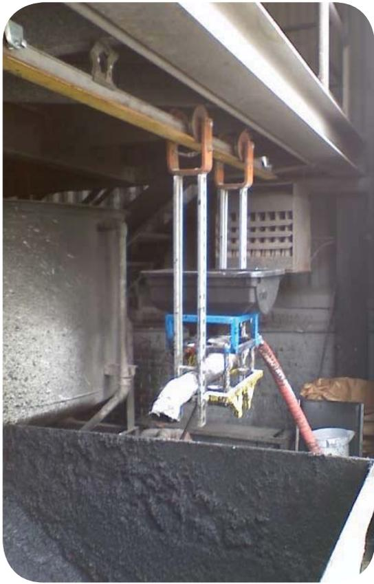
LiquiSorb feeder mounted on overhead monorail
